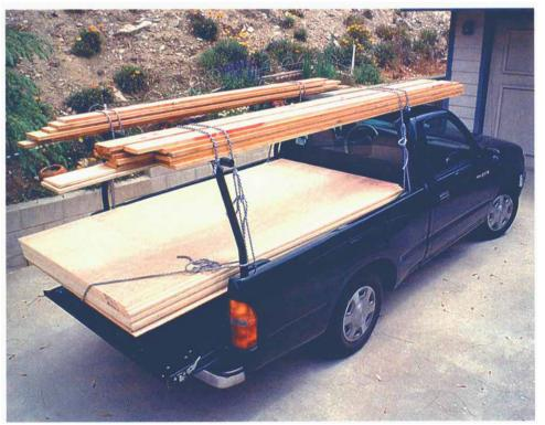
**Two-level rack has sturdy construction and a flexible design.** Simple construction and adaptability make this rack ideal for a small truck. Removing the lower bars or the entire rear unit gives options when hauling large loads.
