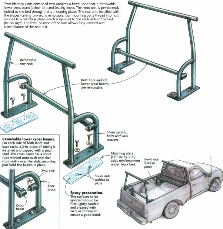
I also noted the wheel-well height and added a couple of inches when I specified the height for the removable lower bars. The crossbars overhang 4 in. on each side to give back the width that's been sacrificed in the interest of matching the slope of the cab.
